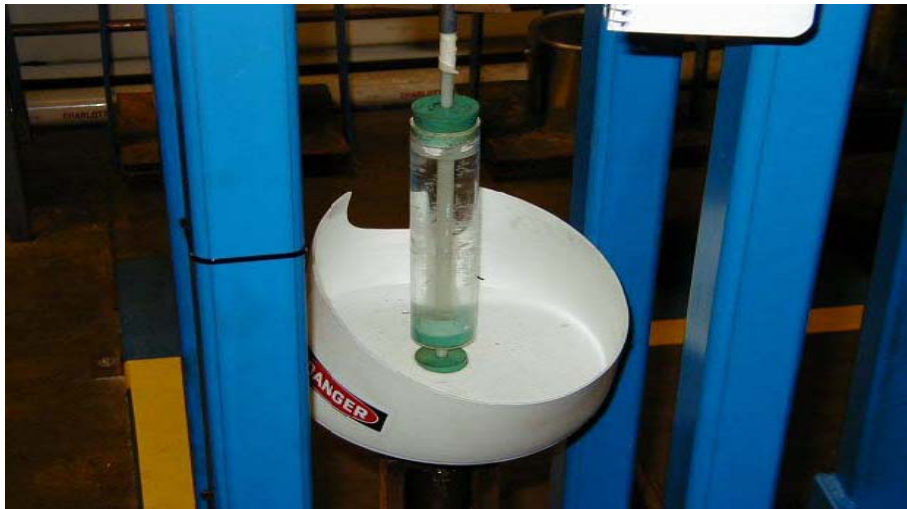
Figure 5 Strained rod immersed in water. (Courtesy Owens Corning)
