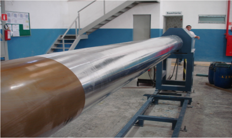
Fig 2. Shows the metal foil wrapped over the mandrel
