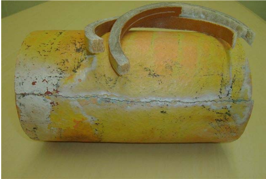
Figure 3 Showing the strain corroded invert of a pipe that operated deflected by vertical compressive loads while carrying an acidic solution. The strain-corrosion process typically ruptures the composite along a neat and well defined smooth surface, instead of the jagged and splintered surface typical of other modes of rupture. Notice that the liner away from the pipe invert was hardly affected by the environment. The crack initiated and progressed from the inside of the pipe.
